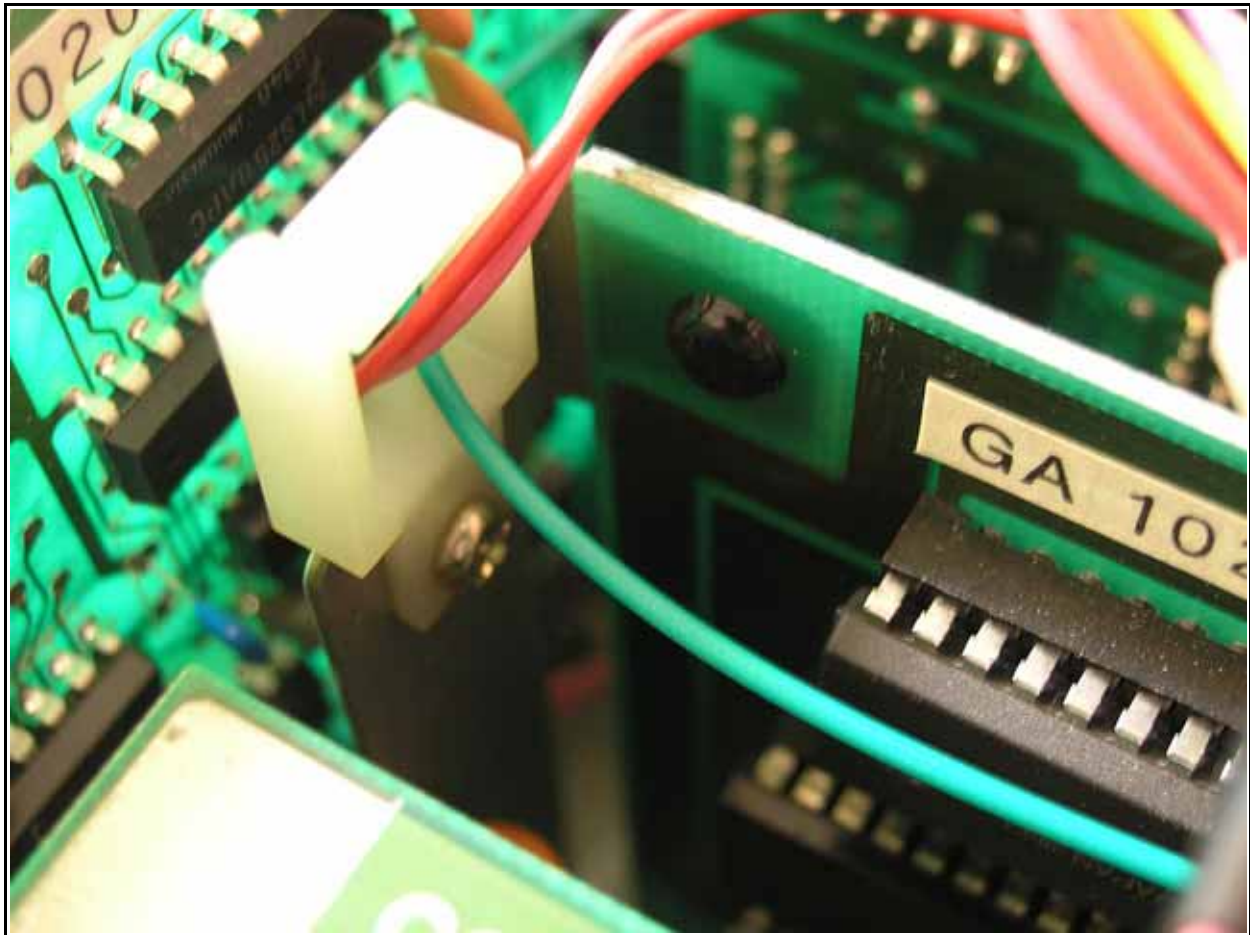
Figure 35 – Route green wire through wire loom to the left side
