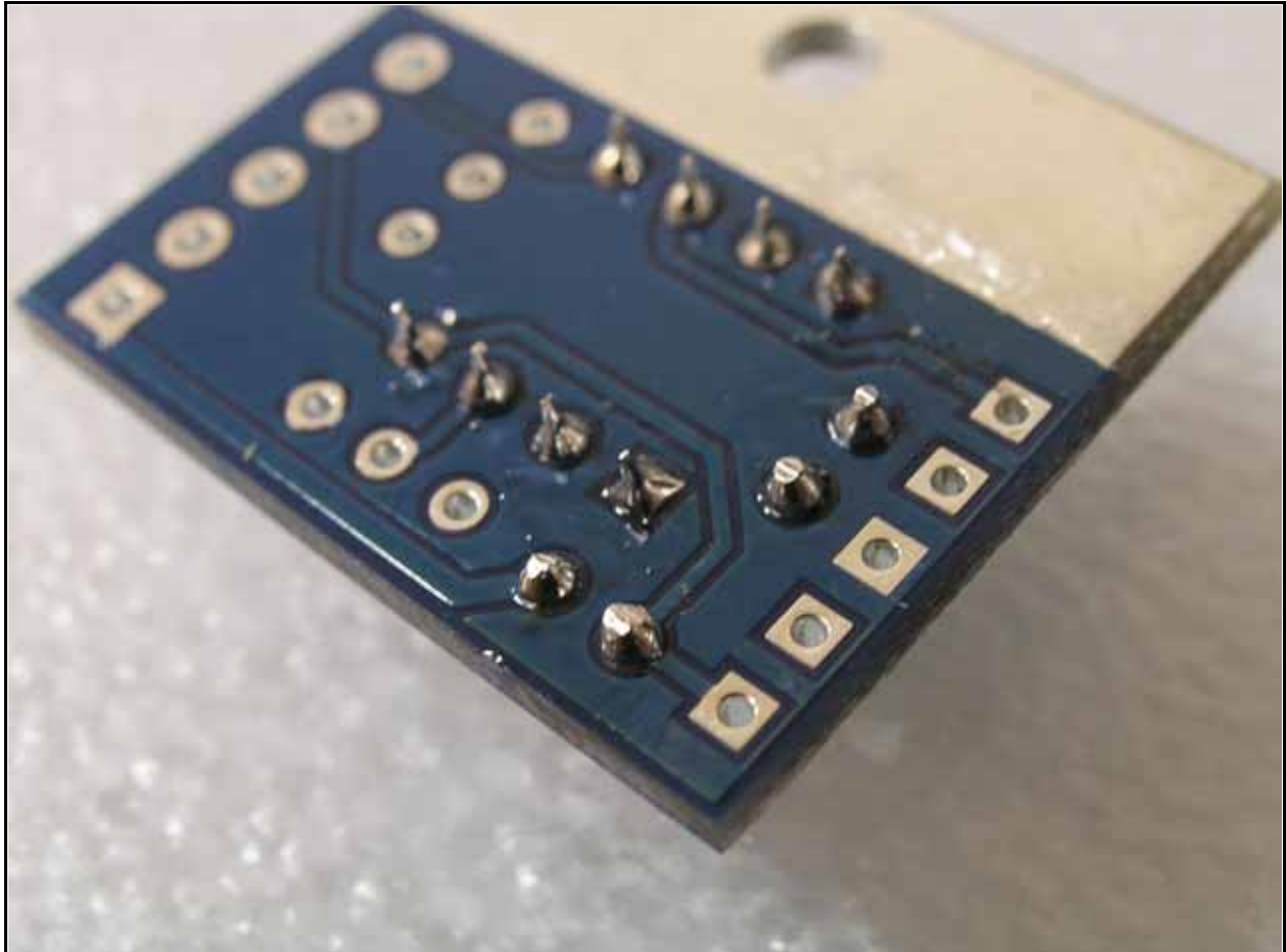
Figure 9 – Resistor soldered and leads cut flush
