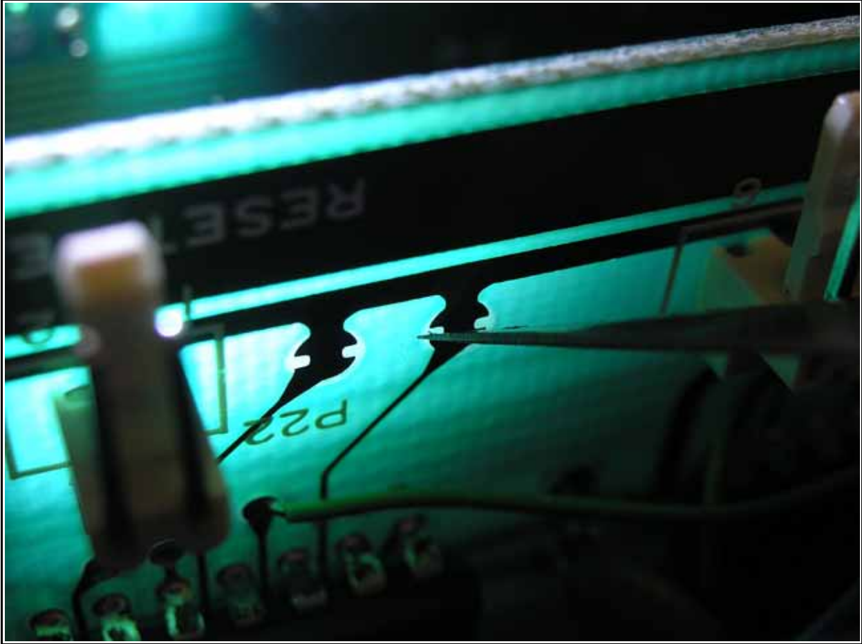
Figure 30 – Positioning the blade of the knife
