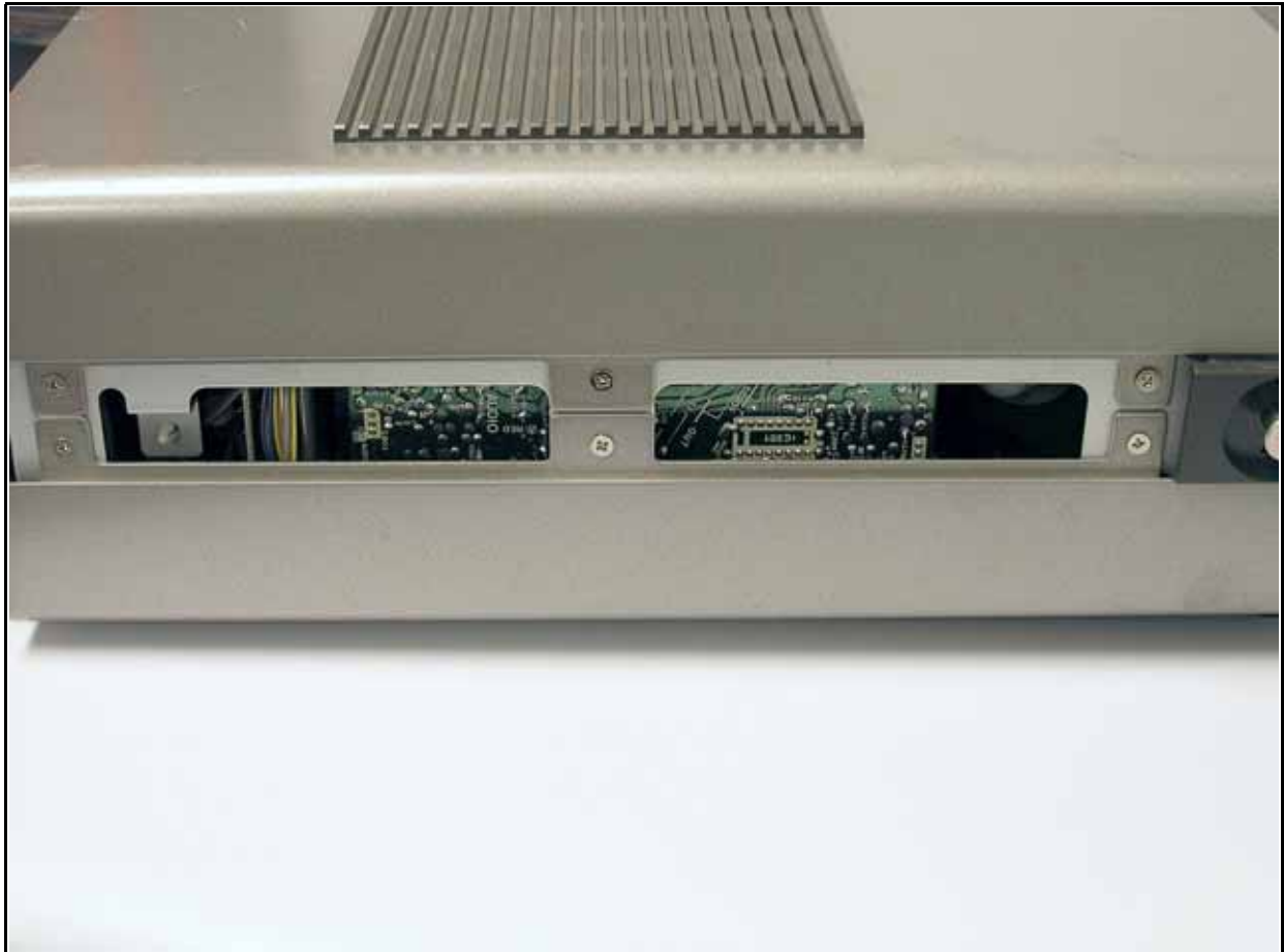
Figure 18 – Location of side screws – remove only top screws!
