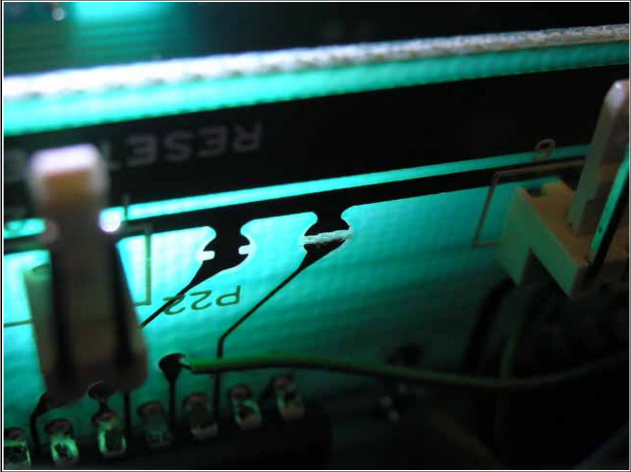
Figure 31 – Pad after being cut apart with knife
