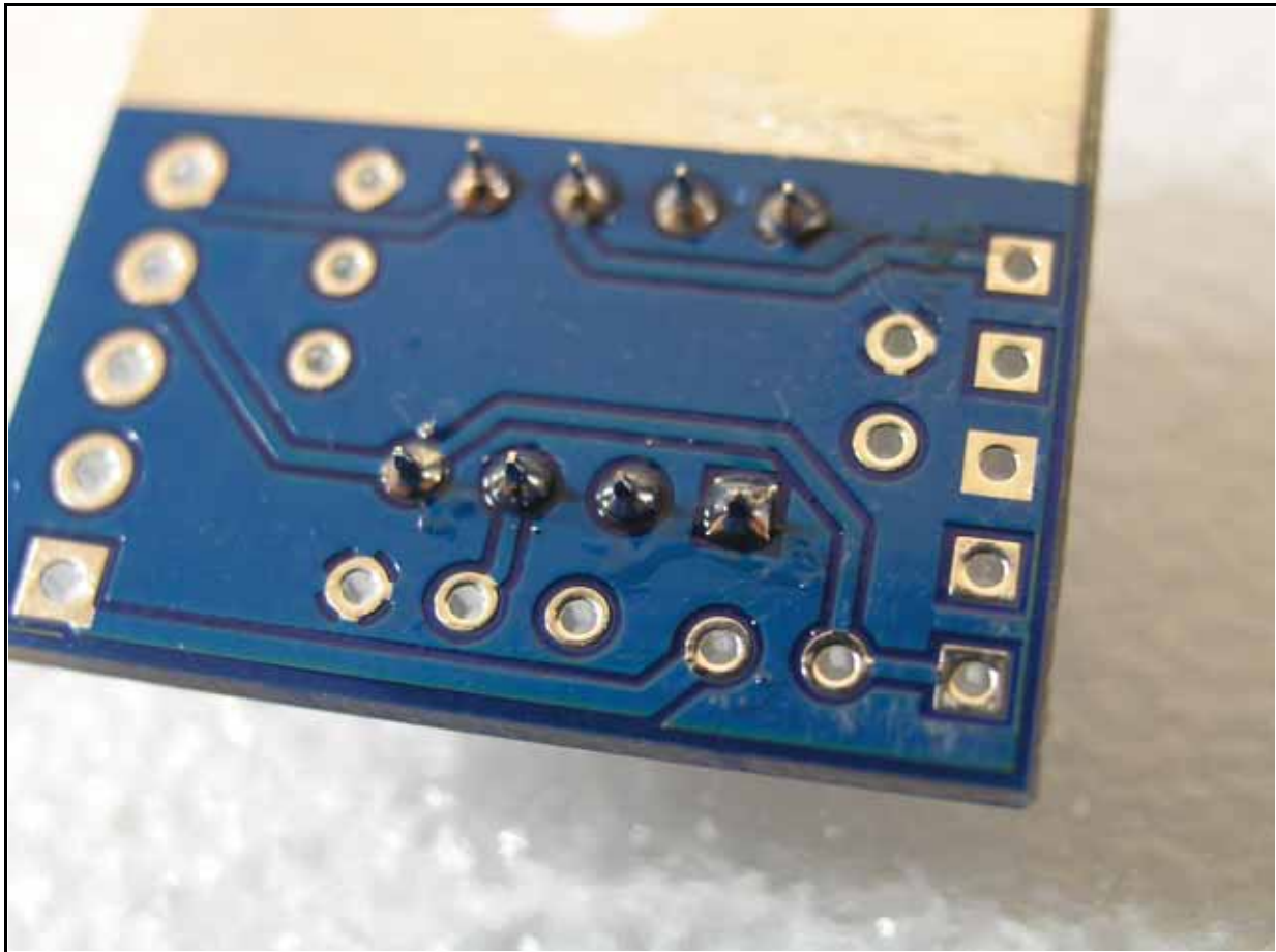
Figure 4 – PIC12F629 soldered in place
