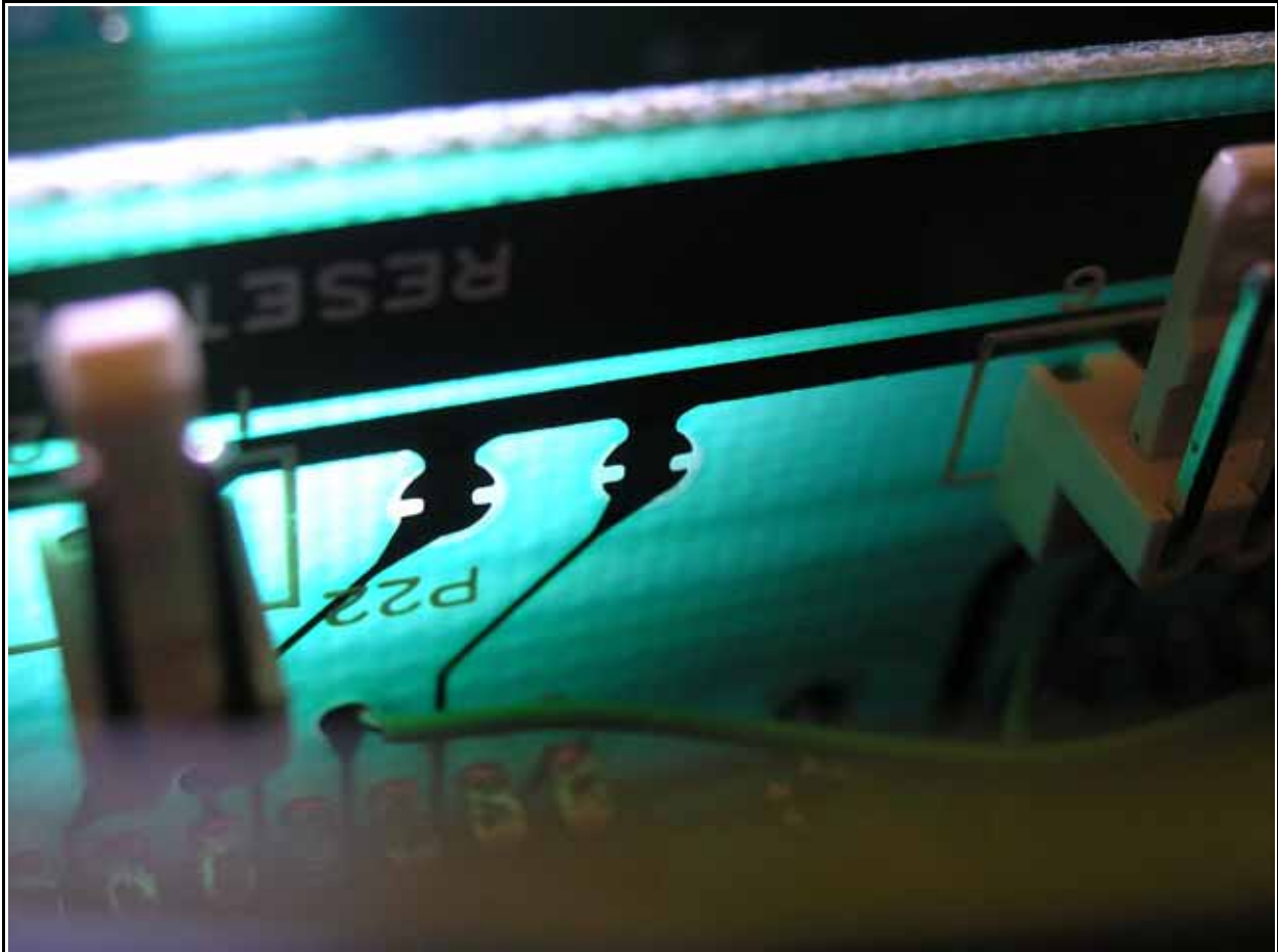
Figure 29 – Back-light makes it easy to see the pads
